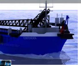
ABEKO Marine received new requests for dredging and land reclamation projects, for which the company had to expand the fleet on the short term with a new trailing suction hopper dredger. Suitable second hand dredgers were not available which made the company decide for the conversion of the MV 'Sirocco', a general cargo vessel built by Barkmeijer Shipyards, into a state-of-the-art Trailing Suction Hopper Dredger.
