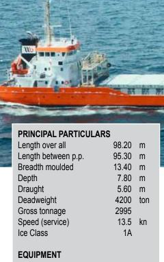
Main engine 2642 kW 315 kW Shaft generator Auxiliary engines (2x) 140 kW Bow thruster 250 kW
