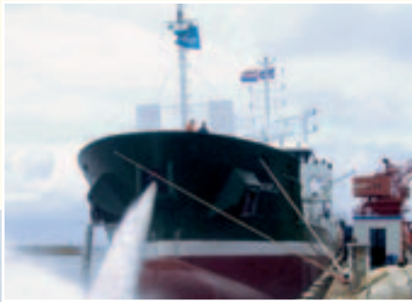
Testing of the discharge systems, either through a discharge line on portside or via a bow coupling.
