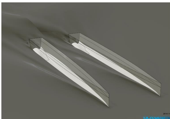
Hull shape and hull spacing were optimised to reduce the wave pattern and required power at 18 knots, as shown here for an intermediate hull-form. Pictures and CFD analysis by Van Oossanen.
