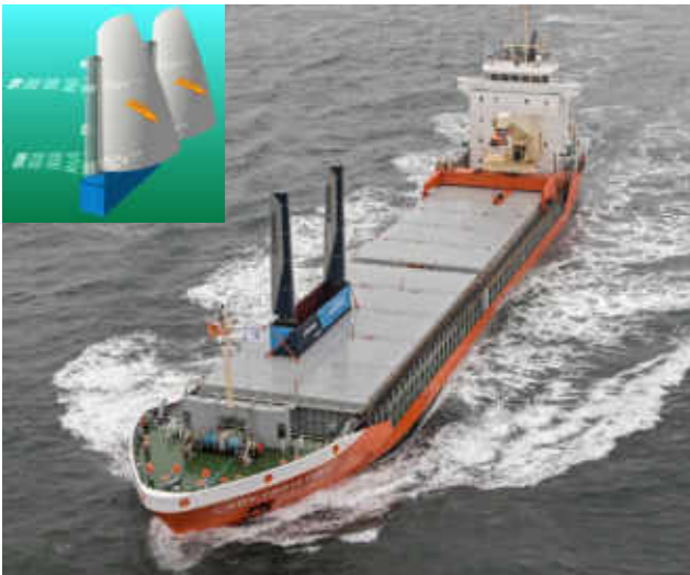
Fig.1: Equal sail-area for identical VentiFoil thrust of one (1) unit
