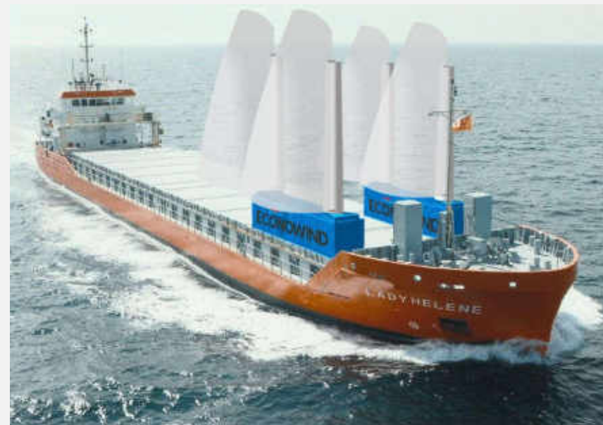
For equivalent thrust force, a sail area of abt. 165 m 2 should be applied !
