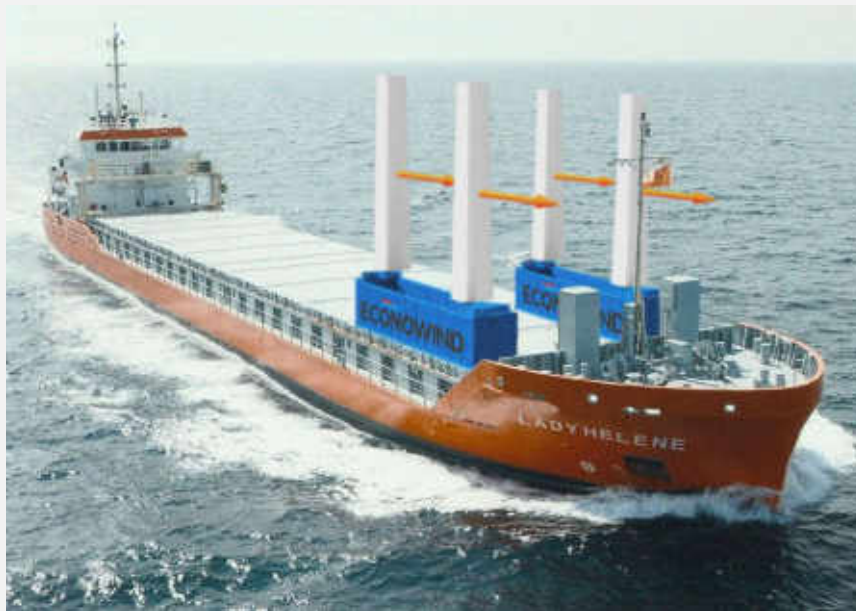
eConowind unit with 2 VentiFoil: Optimal thrust force in compact unit
