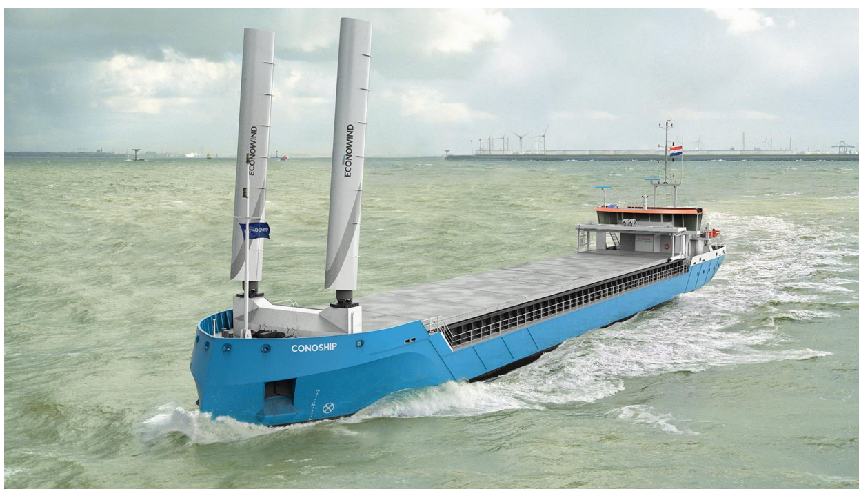
CIP3600 General Cargo Vessel with diesel-electric propulsion | copyright Conoship International
